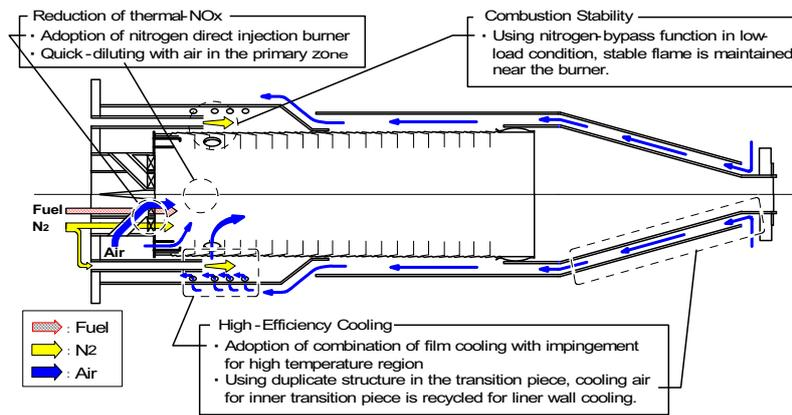
Fig. 17 Design concepts of medium-Btu fueled combustor for wet-type synthetic gas cleanup
