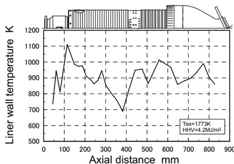
Fig.16 Combustor wall temperature distribution
