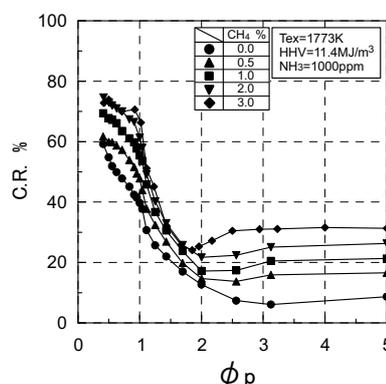
Fig.24 Effect of the  $\text{CH}_4$  concentration on conversion rate of  $\text{NH}_3$  to NOx in two-stage combustion of medium-Btu fuel
