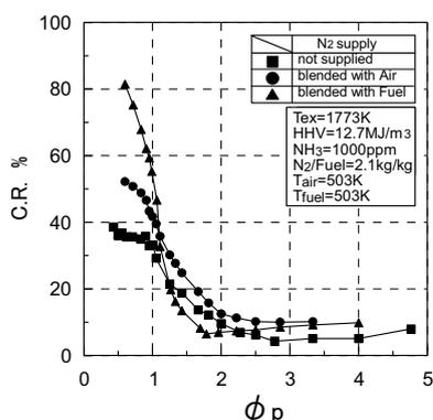
Fig.23 Effect of nitrogen injection on the conversion rate of  $\text{NH}_3$  to NOx in two-stage combustion, using a small diffusion burner
