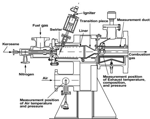
Fig.14 Combustion test rig
