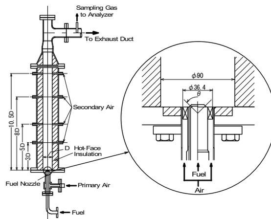
D : inner diameter of cylinder-style combustion chamber, 90mm
