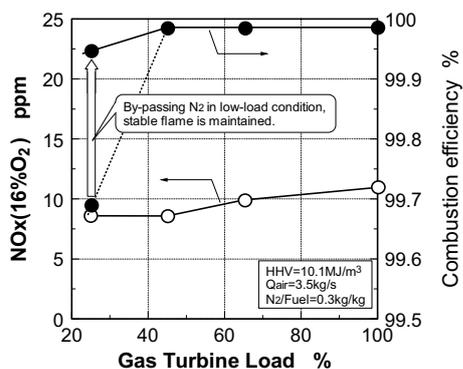
Fig.20 Effect of the gas turbine load on combustion emission characteristics
