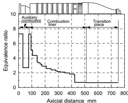
Fig.22 Axial distribution of equivalence ratio at the rated load condition
