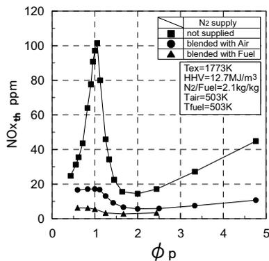
Fig. 18 Effect of nitrogen injection on thermal-NO<sub>x</sub> emission characteristics in two-stage combustion, using a small diffusion burner
