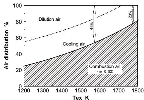
Fig.8 Air distribution design of a gas turbine combustor that burns low-Btu gasified coal fuel
