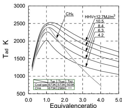
Fig.7 Relationship between equivalence ratio and adiabatic flame temperature for gasified coal fuels and CH<sub>4</sub>
