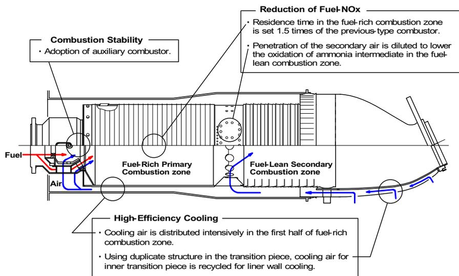
Fig.9 Design concept of 1773K-class low-Btu fueled combustor
