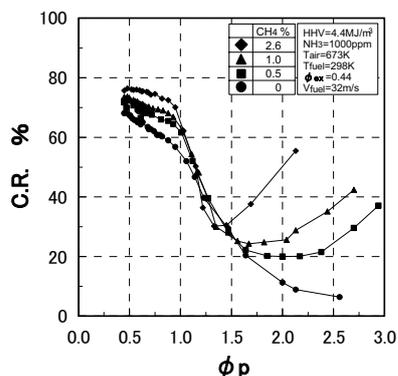
Fig.12 Effect of methane content on conversion rate of ammonia in the fuel to NO<sub>x</sub>, defining by the experiments using a small diffusion burner (Hasegawa et al., 2001)
