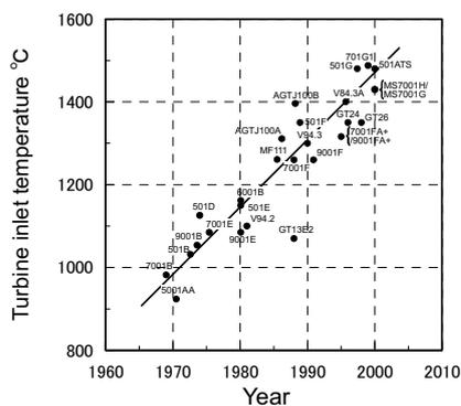
(Signs in figure show names of gas turbine models)
