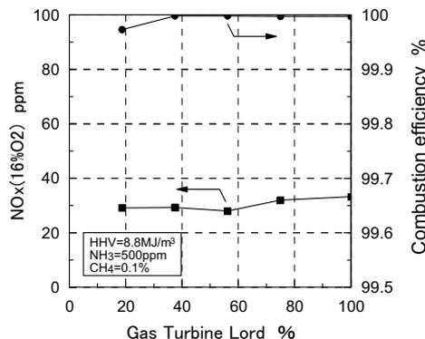
Fig.25 Combustion emission characteristics
