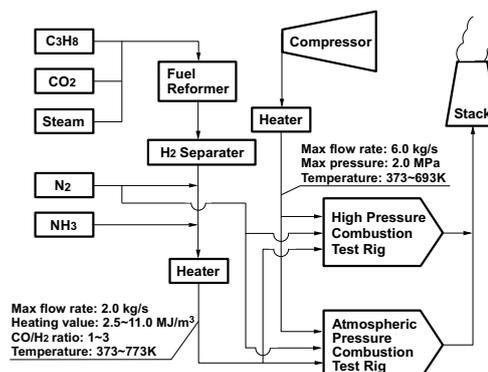
Fig.13 Schematic diagram of test facility
