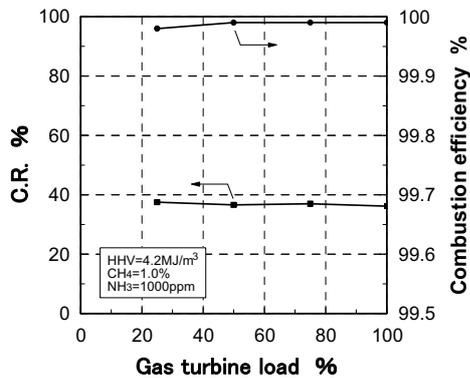
Fig. 15 Combustion emission characteristics
