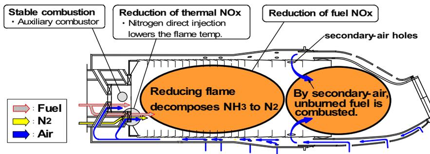
Fig.21 Design concept of a medium-Btu fueled gas turbine combustor for hot/dry-type synthetic gas cleanup
