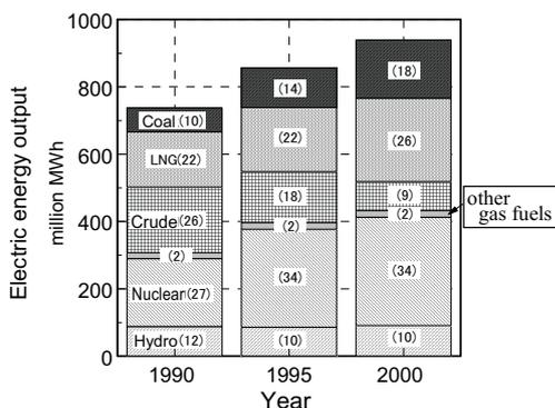
(Numerical value in parentheses shows constituent ratio %) Fig.4 Transition of composition ratio for electric power generation in Japan
