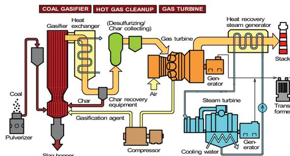
Fig.5 Schematic diagram of typical IGCC system
