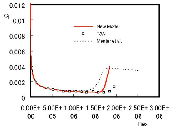
Figure 3 Surface skin friction coefficients for the T3A- case, showing the comparison among the experimental data and two calculated results
