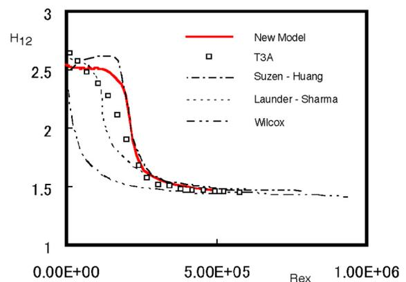
Figure 2 Shape factors for the T3A case, showing the comparison among the experimental data and several calculated results
