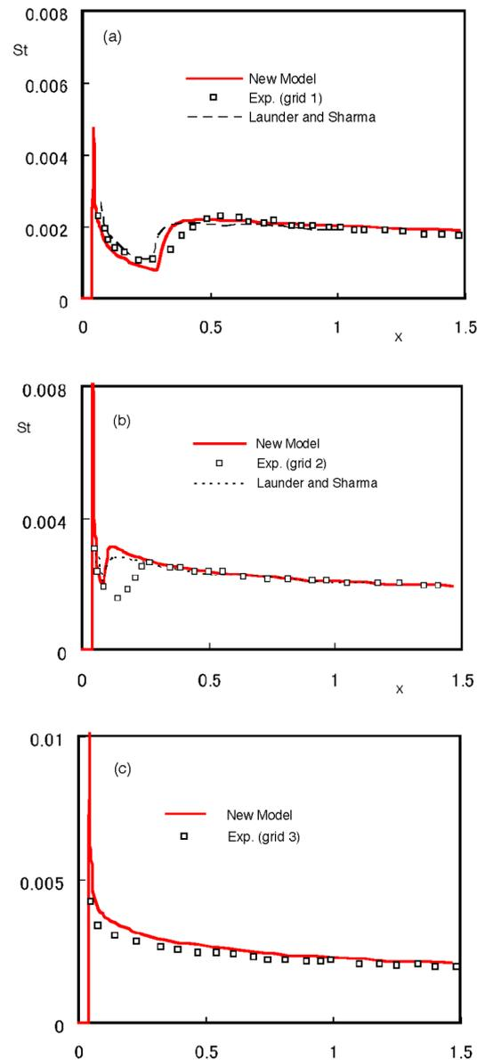
Figure 5 Stanton numbers for the Blair and Werle flat plate case with grid 1 ((a)), grid 2 ((b)) and grid 3 ((c)) under no pressure gradient
