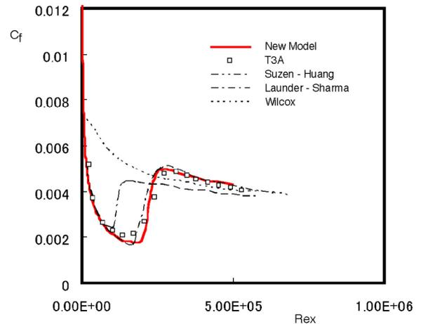
Figure 1 Surface skin friction coefficients for the T3A case, showing the comparison among the experimental data and several calculated results
