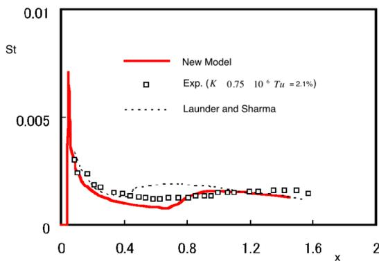
Figure 6 Stanton numbers for the Blair and Werle flat plate case under favorable pressure gradients
