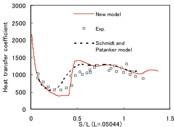
Figure 7 Heat transfer coefficients on the suction side of Daniel and Browne turbine blade
