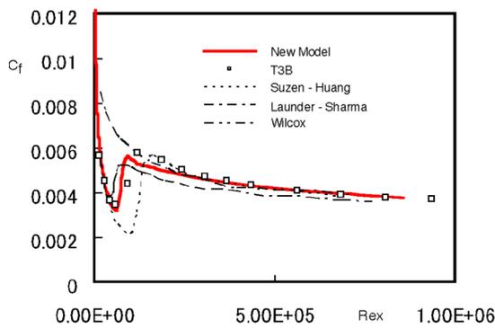
Figure 4 Surface skin friction coefficients for the T3B case, showing the comparison among the experimental data and several calculated results
