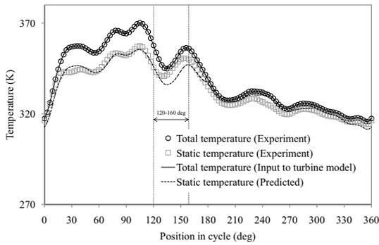
Figure 9: Predicted instantaneous temperature profile under 60 Hz pulsating inflow
