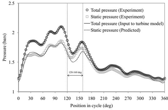
Figure 8: Predicted instantaneous pressure profile under 60 Hz pulsating inflow
