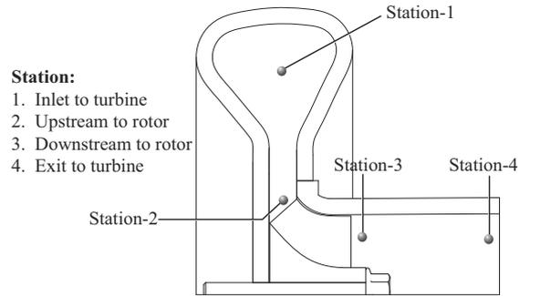
Figure 2: Turbine Station 1, Station 2, Station 3 and Station 4 [4]
