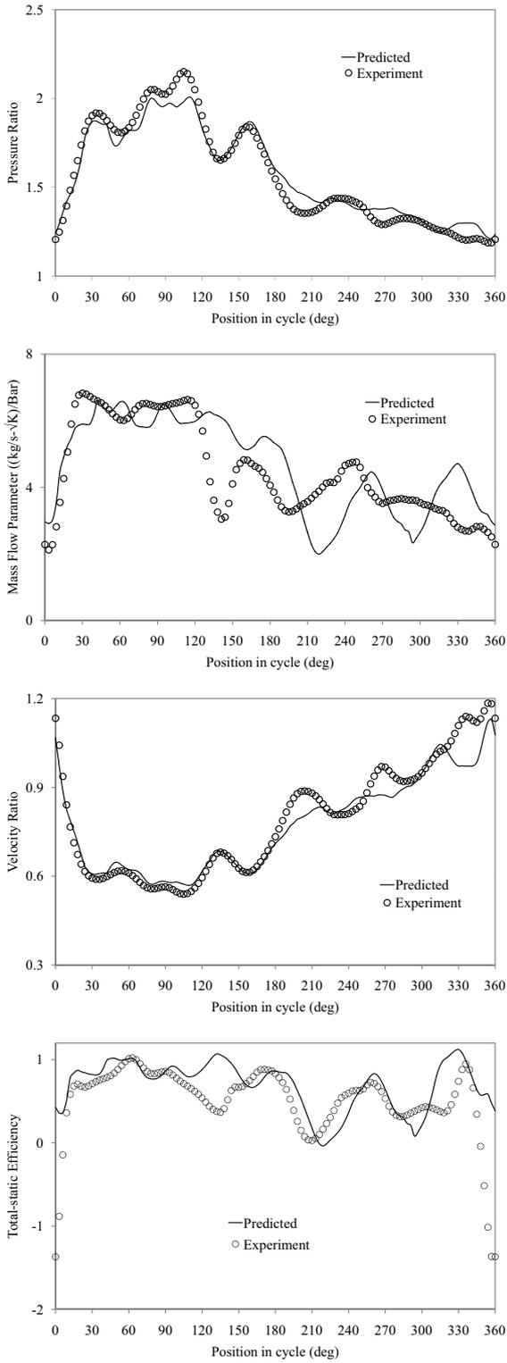
Figure 12: Predicted pressure ratio, mass flow parameter, velocity ratio and efficiency against pulse cycle
