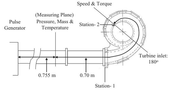
Figure 1: Mean flow path throughout turbine and illustration of turbine Station 1 & 2 [3]
