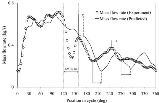
Figure 10: Predicted instantaneous mass flow rate profile under 60 Hz pulsating inflow with illustration of out-of-phase predicted mass flow peak with corresponding experimental peak
