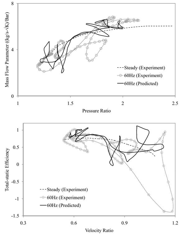
Figure 13: Predicted mass flow parameter-pressure ratio and efficiency-velocity ratio
