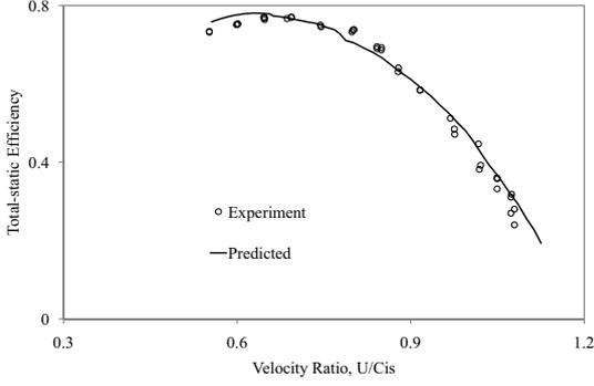
Figure 7: Predicted steady state turbine efficiency
