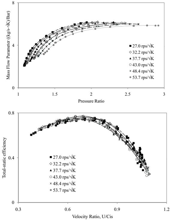
Figure 3: Steady state mass flow parameter and turbine efficiency at 27.0 – 53.7 rps/√K turbine speed [3]
