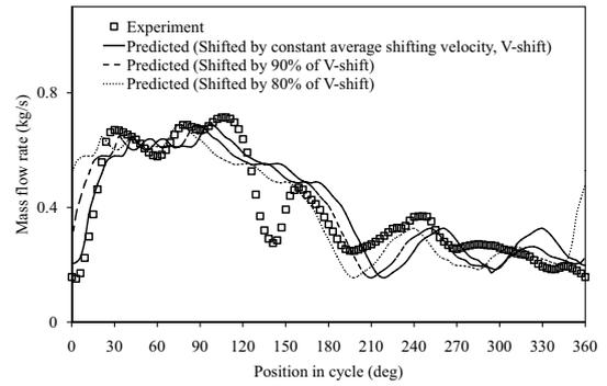
Figure 11: Phase shifting of predicted mass flow rate profile with different shifting velocities
