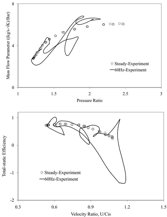
Figure 4: Turbine mass flow parameter and efficiency under 60Hz pulsating flow at 43.0 rps/√K turbine speed [3]
