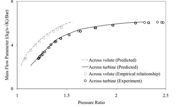
Figure 6: Predicted MFP-PR across stator and turbine
