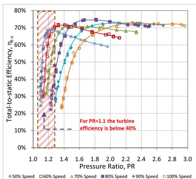
Figure 1: Mixed-flow turbine performance
