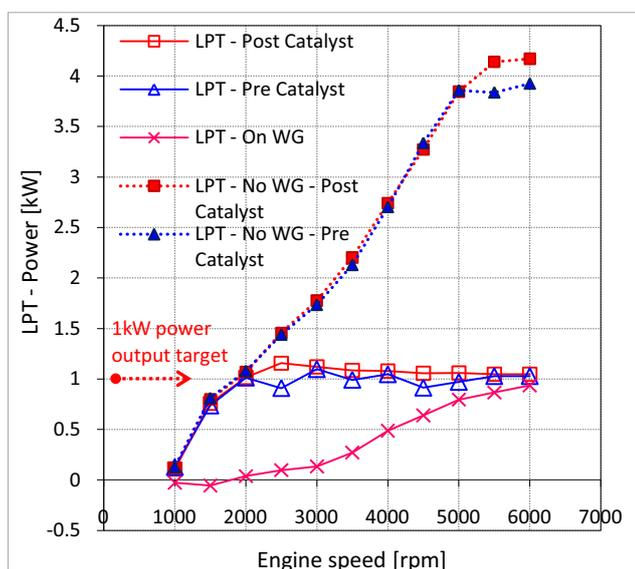
Figure 11: Power output for the LPT at 50000 rpm: comparison with the case where no constraint is set on max power.
