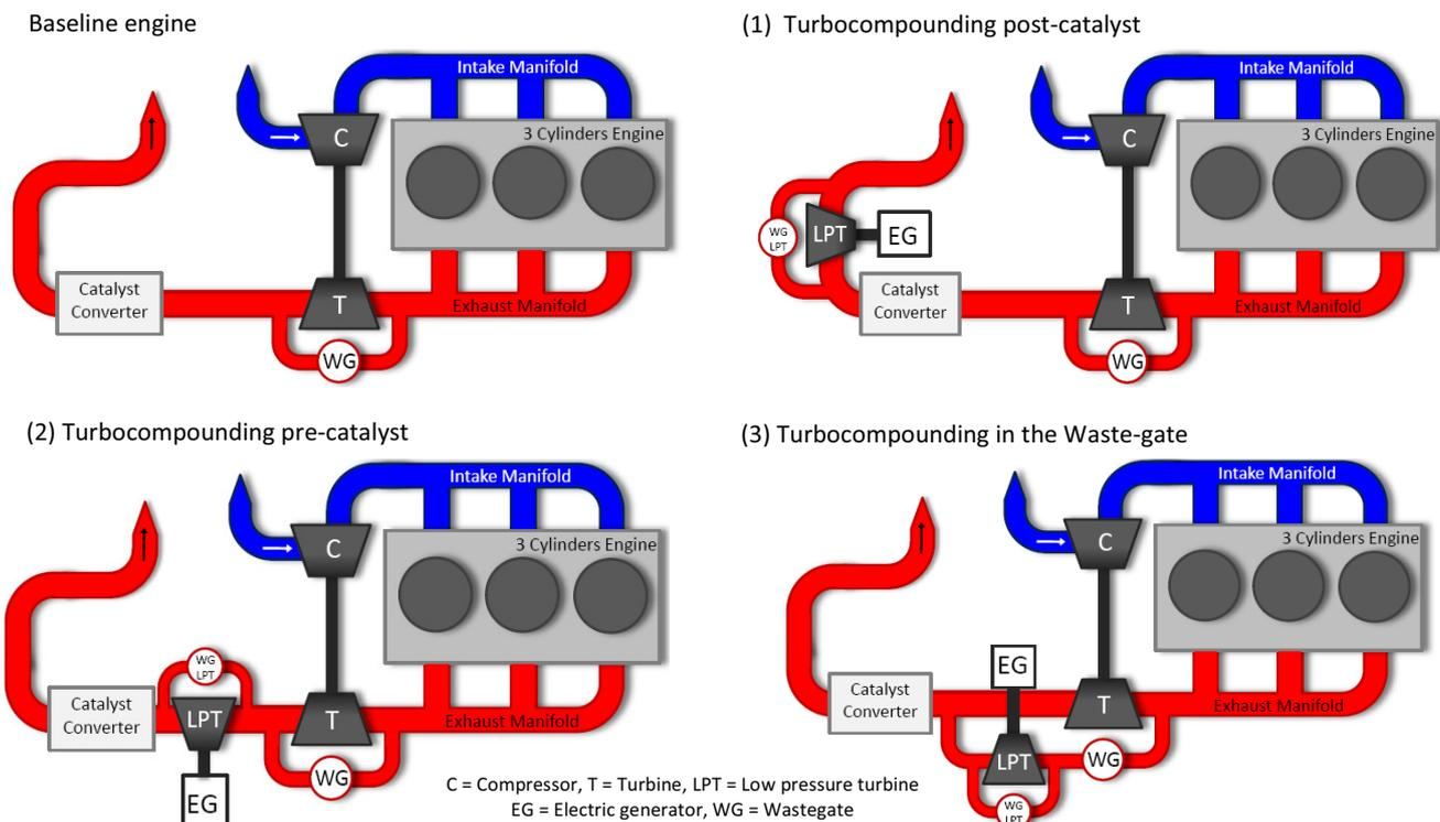
Figure 9: Positions of the low pressure turbine (LPT) as compared with the baseline engine
