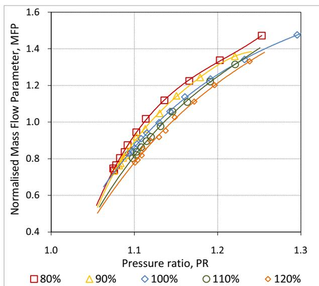
Figure 7: Normalised MFP vs. PR for cold-flow test
