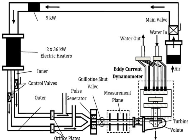
Figure 4: Imperial College cold-flow test facility
