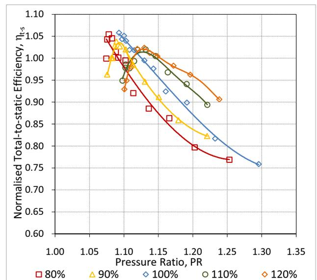
Figure 5: Normalised  $\eta_{t-s}$  vs. PR for cold-flow test
