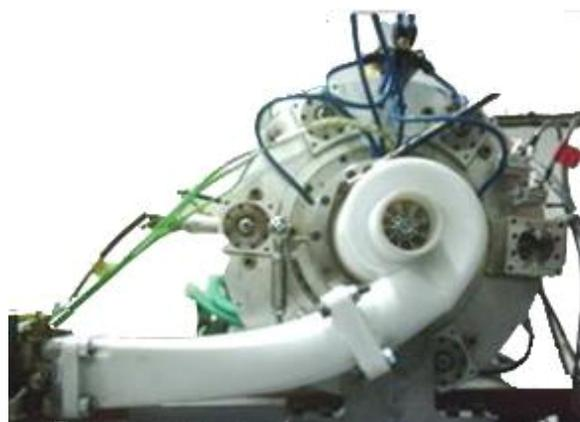
Figure 3: LPT installed in the Imperial College cold-flow test facility
