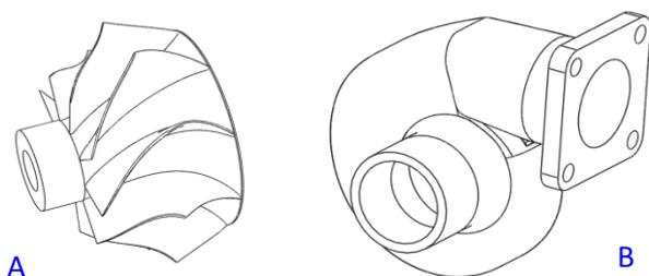
Figure 2: Low pressure turbine, 3-D view of the turbine wheel (A) and volute (B)
