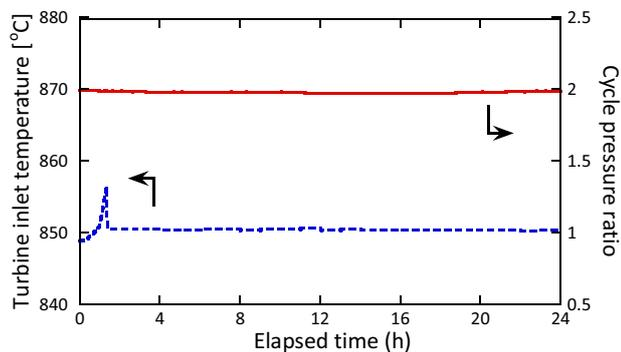
Fig.23 Transient response of turbine inlet temperature and cycle pressure ratio during the load-following operation for Jeddah
