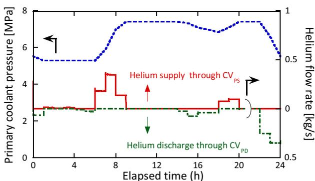
Fig.12 Transient response of primary coolant pressure and flow rate at primary helium supply flow rate control valve during the load-following operation for Almaty
