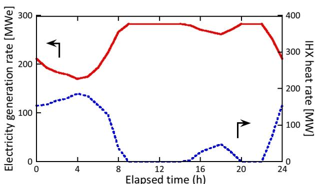
Fig.13 Transient response of electricity generation rate and IHX heat rate during the load-following operation for Almaty
