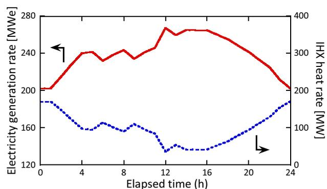
Fig.20 Transient response of electricity generation rate and IHX heat rate during the load-following operation for Jeddah
