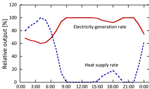
Fig.11 Scheduled load curve for load-following operation in Almaty
