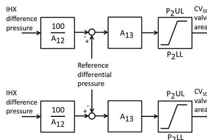
Fig.8 Block diagram of IHX differential pressure controller
