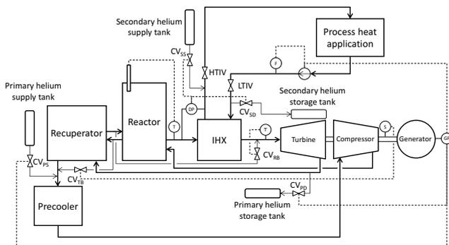
Fig.3 Basic control scheme of the GTHTR300C
