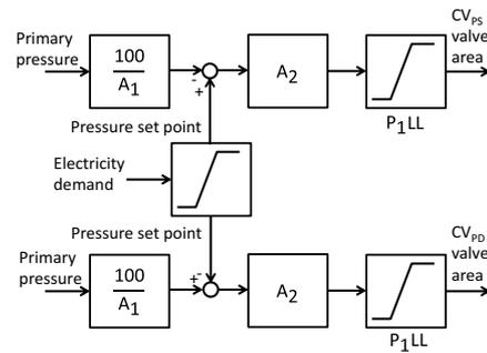
Fig.4 Block diagram of inventory controller
