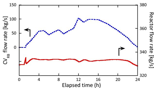
Fig.21 Transient response of flow rate at reactor bypass flow rate control valve and reactor flow rate during the load-following operation for Jeddah
