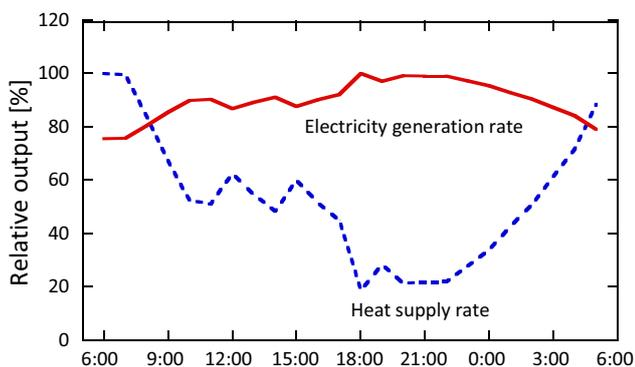
Fig.18 Scheduled load curve for load-following operation in Jeddah
