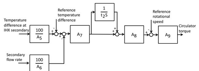
Fig.6 Block diagram of IHX heat rate controller
