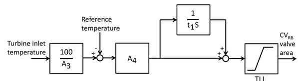
Fig.5 Block diagram of turbine inlet temperature controller
