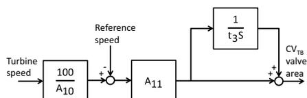
Fig.7 Block diagram of turbine speed controller
