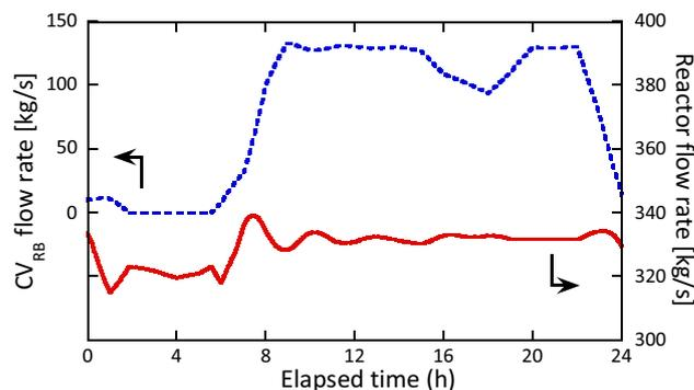
Fig.15 Transient response of flow rate at reactor bypass flow rate control valve and reactor flow rate during the load-following operation for Almaty
