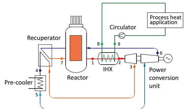
Fig.1 Schematic layout of the GTHTR300C
