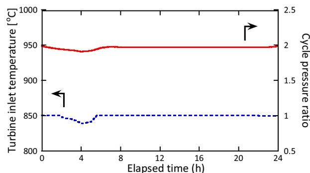
Fig.14 Transient response of turbine inlet temperature and cycle pressure ratio during the load-following operation for Almaty
