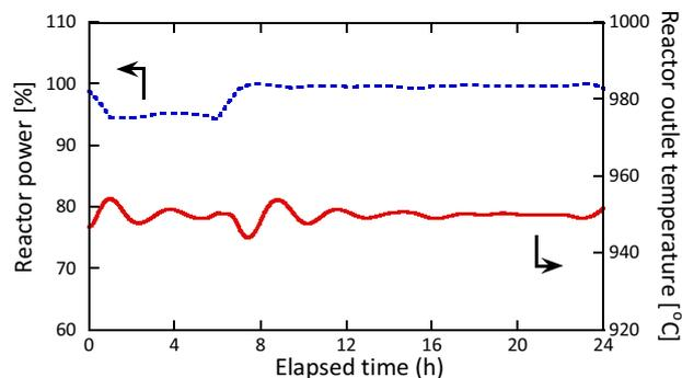
Fig.16 Transient response of reactor power and reactor outlet temperature during the load-following operation for Almaty
