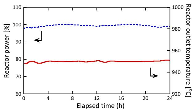
Fig.22 Transient response of reactor power and reactor outlet temperature during the load-following operation for Jeddah
