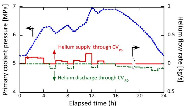
Fig.19 Transient response of primary coolant pressure and flow rate at primary helium supply flow rate control valve during the load-following operation for Jeddah
