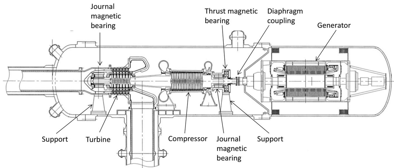
Fig.2 Horizontal view of the GTHTR300C power conversion unit [5]
