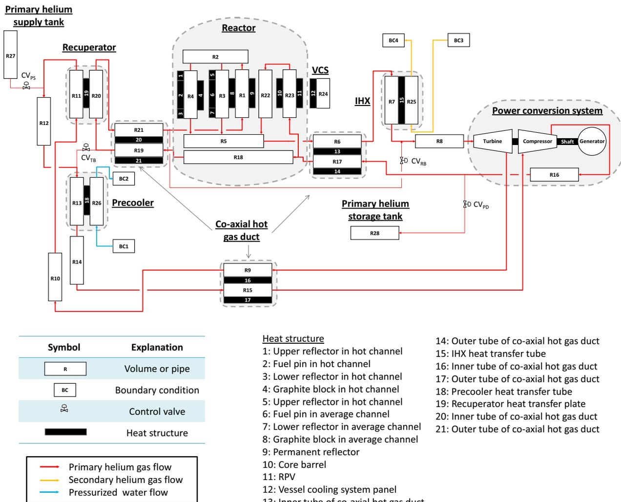
Fig.9 Nodalization of GTHTR300 model
