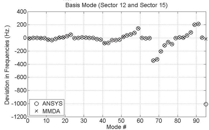
Figure 5: Deviations in natural frequencies estimated via full rotor FEM and MMDA (Alternative Bases, Sectors 12 and 15)
