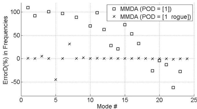
Figure 12: Errors (%) in deviations of natural frequencies estimated via MMDA (POD 1 only) and MMDA (POD 1 and rogue blade)
