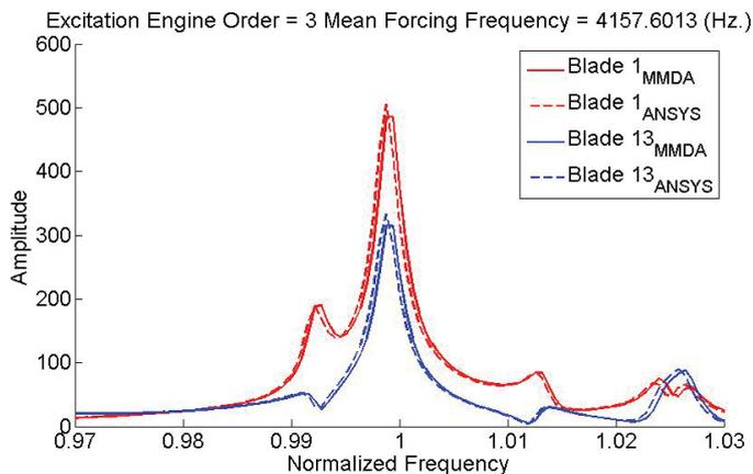
Figure 10: Blade tip amplitude estimated via full rotor ANSYS and MMDA (Alternative Basis, Sector 4 and 23), 3EO excitation
