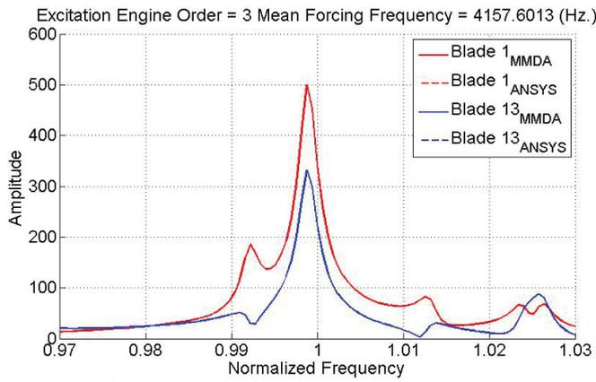
Figure 7: Blade tip amplitude estimated via full rotor ANSYS and MMDA (Alternative Basis, Sectors 12 and 15) for 3EO excitation
