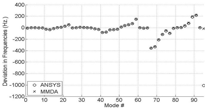
Figure 9: Deviations in natural frequencies estimated via full rotor ANSYS and MMDA (Alternative Bases, Sectors 4 and 23)
