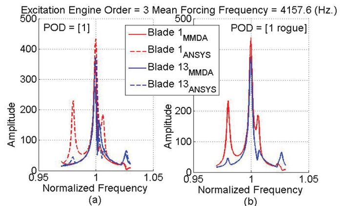
Figure 13: Blade tip amplitude estimated via full rotor ANSYS, MMDA (POD 1 only) and MMDA (POD 1 and rogue blade) for 3EO excitation
