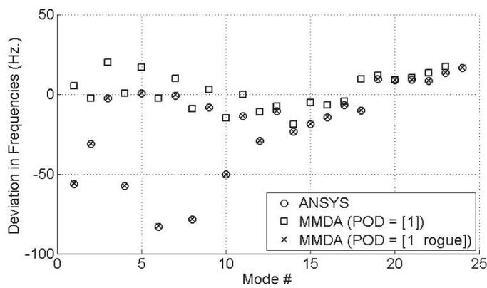
Figure 11: Deviations in natural frequencies estimated via full rotor ANSYS, MMDA (POD 1 only) and MMDA (POD 1 and rogue blade)
