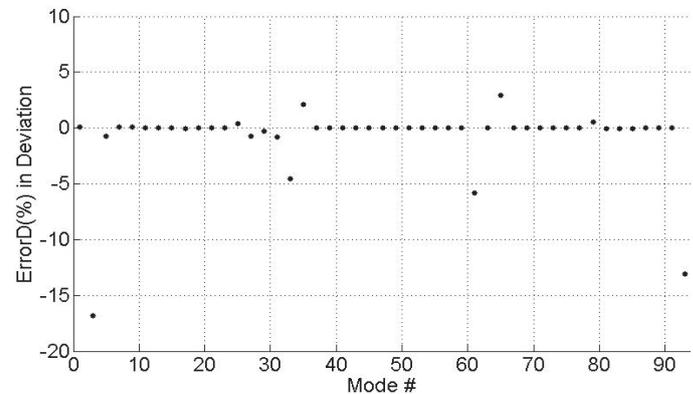
Figure 6: Errors (%) in deviations of natural frequencies estimated via MMDA (Alternative Bases, Sectors 12 and 15)
