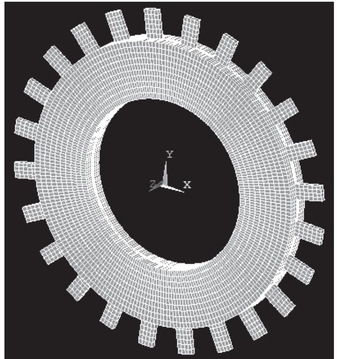
Figure 1: Finite element model of the academic rotor (Sinha, 2009)
