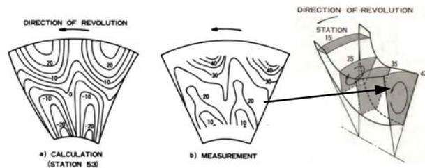
Fig. 5 Radial turbine flow measurement
