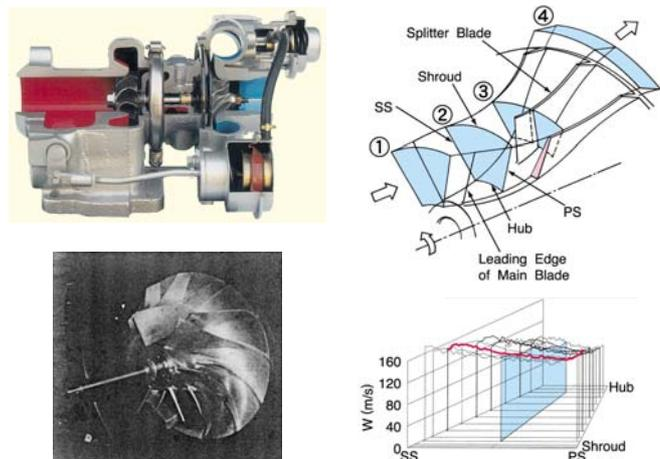
Fig. 1 Passenger car turbocharger, and LDV measurement for a large scale model of an actual impeller
