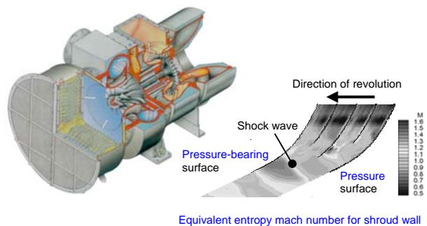
Fig. 2 Marine diesel engine turbocharger, and pressure measurement for shock wave generation
