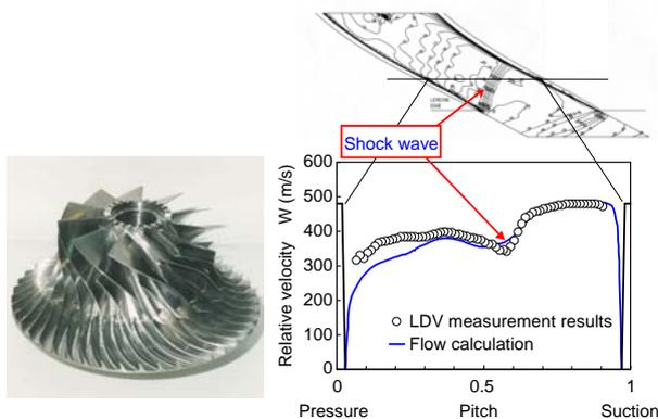
Fig. 4 High pressure ratio impeller and shock wave measurement
