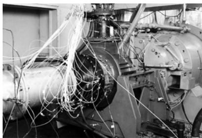
Fig. 3 Gas turbine compressor test facility
