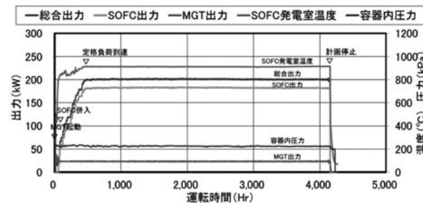
Fig. 10 Long term behavior of model 10 SOFC-MGT hybrid system installed at Tokyo Gas Co.,Ltd.'s Senju Techno Station (It was provided by MHPS)
