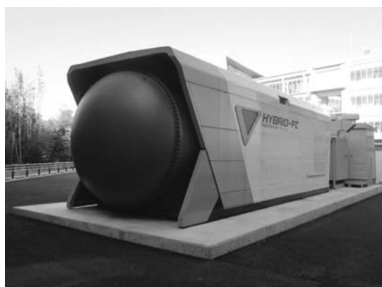
Fig. 12 Appearance of model 15 SOFC-MGT hybrid system installed at the Next-Generation Fuel Cell Research Center (NEXT-FC) in Kyushu University (It was provided by MHPS)
